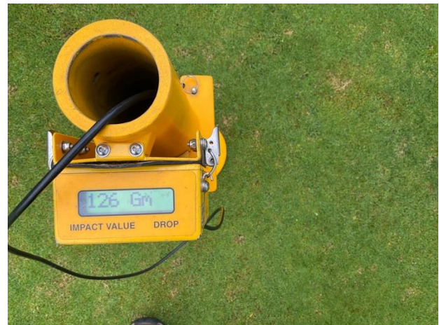
Photo 4: In the same corner, a very encouraging surface firmness of 126 gravities was recorded on the morning of the visit.
