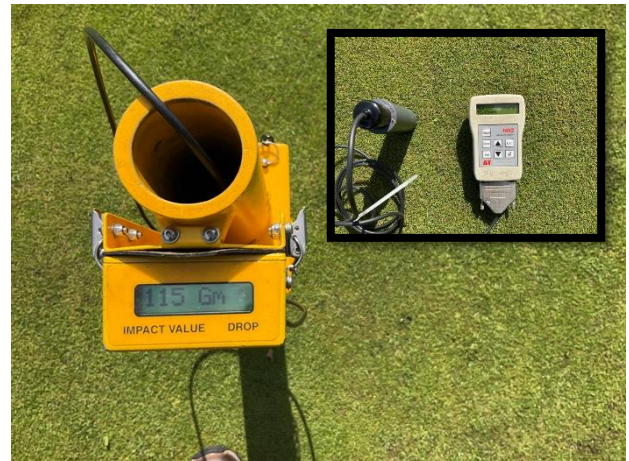
Figure 22: Water content remains higher than desirable at 35.6% (inset), but surface firmness is still an encouraging 115 gravities.
