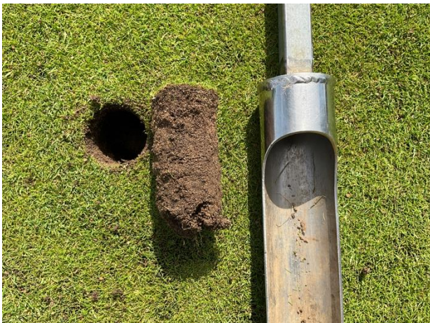
Figure 21: The soil profile displays a relatively shallow rooting network and persistent thatch accumulation in the top 20mm.
