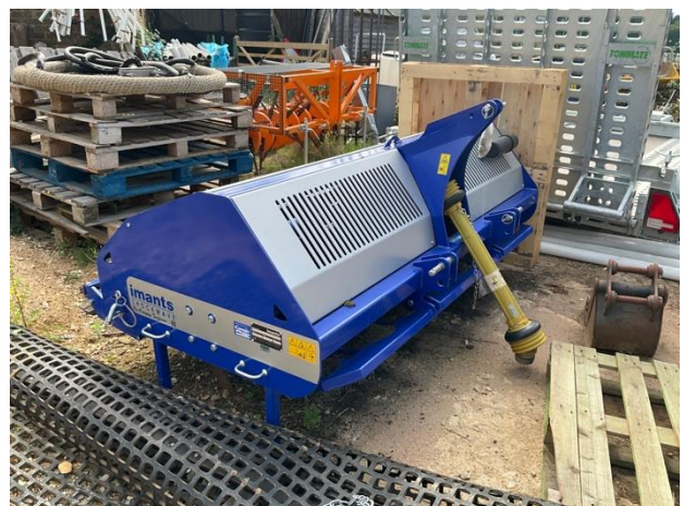
Figure 18: The Imants Shockwave unit should be employed in the “wet” section at West Witney to optimise drainage and improve root extension.
